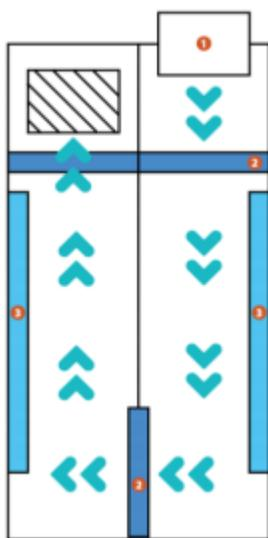
1. Fresh air exhaust fan with a capacity of 540m<sup>3</sup>
